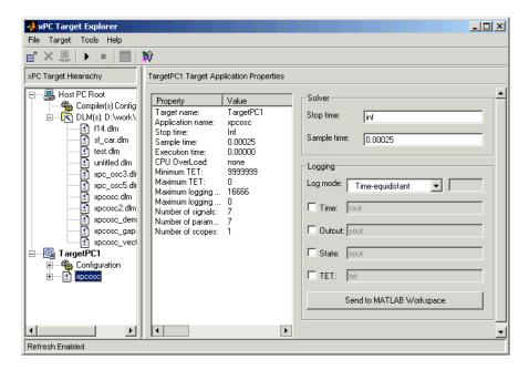
2 To get the list of signals in the target application, expand the target application node, then expand the Model Hierarchy node under the target application node.
