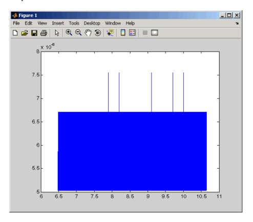
The TET is the time to calculate the signal values for the model during each sample interval. If you have subsystems that run only under certain circumstances, plotting the TET would show when subsystems were executed and the additional CPU time required for those executions.
