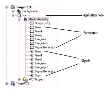
The Model Hierarchy node can have up to three nodes: subsystems () (including their signals and parameters), parameters (), and signals (). Only xPC Target tunable parameters and signals of the application, as represented in the Simulink model, appear in the Model Hierarchy node. This example currently has only parameters and signals.
