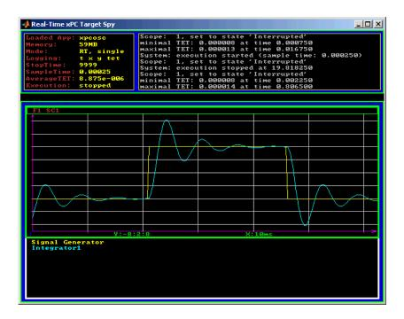
4 Add signals to the host PC scope. For example, to add signals Integrator1 and Signal Generator, right-click each signal and select Add to Scopes. From the Add to Scopes list, select Scope 2.
