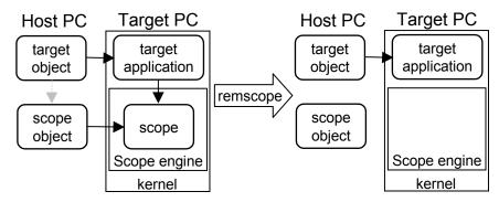
Note that you can only permanently remove scopes that are added with the method addscope. This is a scope that is outside a model. If you remove a scope that has been added through a scope block (the scope block is inside the model), a subsequent run of that model creates the scope again.
