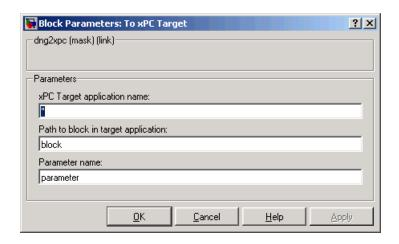
**Note** The use of To xPC Target blocks require a connection between the host and target PC. If there is no connection between the host and target PC, operations such as opening a model that contains these blocks or copying these blocks within or between models, will take significantly longer than normal.
