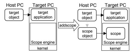
**Scope of type file** — Data collected is stored in a file in the target PC file system. You can then transfer the data to another PC for examination or plotting.
