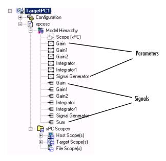
Each signal in the signals section has a corresponding entry in the parameters section. To change the value of a signal, you need to select the corresponding parameter entry. Note that if a parameter is not tunable, it does not appear in the parameter area.
