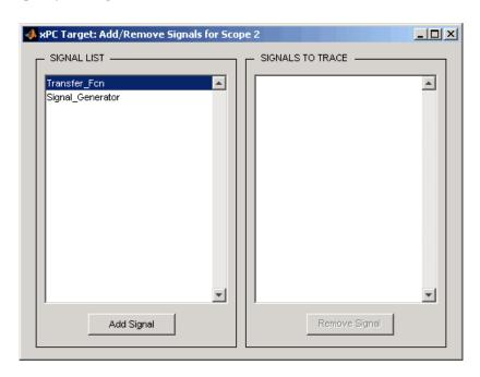
The **SIGNAL** list box displays all the available signals from the target application. The names of the signals shown correspond to the block names within the Simulink model xpc osc4.mdl. The block name indicates the output signal from that block.
