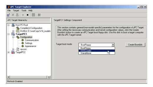
The default setting for the option **TargetBoot** is BootFloppy. When using BootFloppy, xPC Target must first create a target boot disk, which is then used to boot the target PC.
