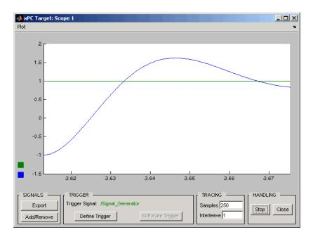
If you are using a scope of type host, there is a delay between collecting data packages because of the communication overhead between the target PC and the host PC. If you are using a scope of type target, the scope window is updated faster than when using a scope on the host PC.
