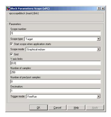
This setting is required to enable target scopes to begin operating as soon as the application starts running. This setting is important because the host PC is not available in StandAlone mode to issue a command to start scopes.
