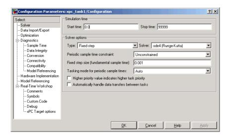
**Note** The user interface model should only contain discrete-time elements, and therefore you should only select the discrete solver. The model should not contain any continuous-time states.
