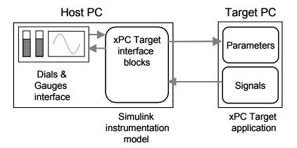
Virtual Reality Toolbox — The Virtual Reality Toolbox enables you to display a Simulink user interface model in 3-D. It provides Simulink blocks that communicate with xPC Target interface blocks. These blocks then communicate with a graphical user interface. This graphical user interface is a Virtual Reality Modeling Language (VRML) world displayed with a Web browser using a VRML plug-in.
