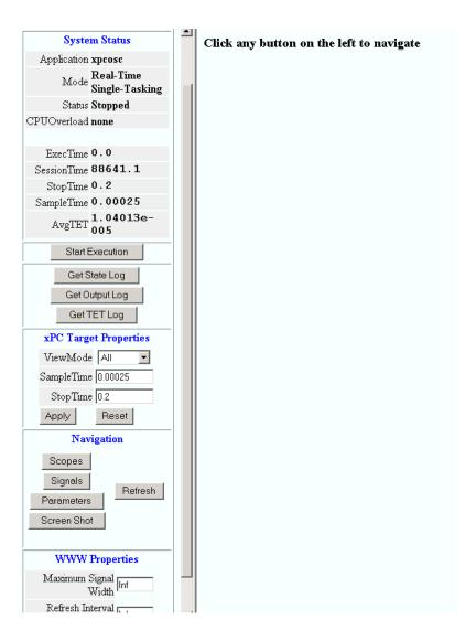
After you connect a Web browser to the target PC, you can use the **Main** pane to control the target application:
