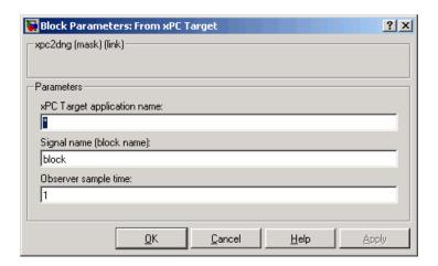
**Note** The use of From xPC Target blocks require a connection between the host and target PC. If there is no connection between the host and target PC, operations such as opening a model that contains these blocks or copying these blocks within or between models, will take significantly longer than normal.
