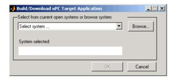
3 From the current open systems list, select the name of a Simulink model (.mdl) you have open, or click the **Browse** button and select the name of a Simulink model or a previously built target application (.dlm). Click **OK**.
