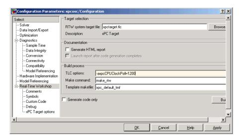
If you want to execute the target application in interrupt mode again, either remove the option or assign a CPU clock rate of 0 to the option:
