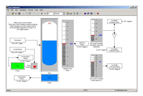
If you do not see the dials and gauges in the Active X blocks, try registering the Active X controls. In the MATLAB window, type
