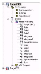
**4** To get the list of scope types you can have in the target application, expand the xPC Scopes node below the application node.
