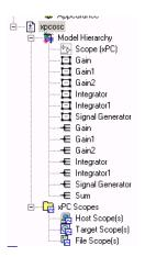
**5** To create a scope to display on the target PC, right-click Target Scopes from the xPC Scopes node.
